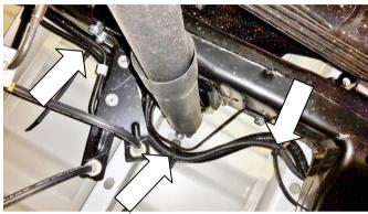
5.9) Cable tie off the wiring loom with 200mm long cable ties in 3 places to the vehicle's wiring loom around the area near the rear shock.
