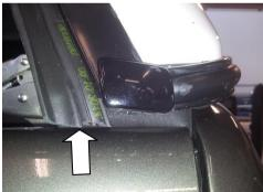
4.8) Cut the lower door gutter seals in line with the top of the tailgate on both sides of the door so they just touch the top of the vehicle's tailgate.
