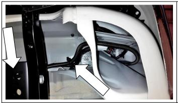
5.5) Cable tie off the wiring loom with a 200mm long cable tie to the vehicle's loom under the RH tail lamp recess underneath the vehicle and another at the chassis rail.
