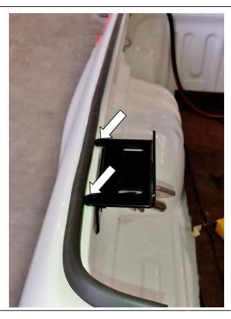
3.1) Align the seal along the sides of the tub by the distance of the tags of the rear canopy mounting brackets. Apply the seal with firm pressure to the tub.
