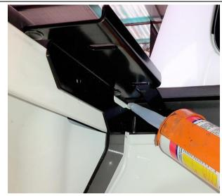
3.8) Apply neutral cure silicon to inside of each end of the "T" section rail top corners. Clean off excess with a rag and silicon remover or wax and grease remover carefully.
