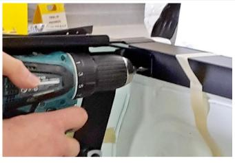
2.9) Drill a 5.2mm holes through the existing 2 holes in the front corner bracket where it touches the "T" section rail extrusion across the front of the tub with a 12mm deep drill stop fitted. Remove any swarf. Apply rust inhibitor (665505) to the drilled holes and insert 2 rivets (6609087). Repeat on other side of tub for the opposite bracket
