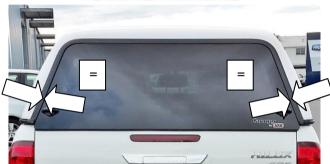
4.1) Align the holes in the base rail so the slots are centred to the rear tub mounting brackets.
