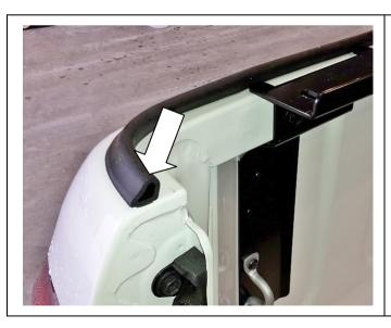
3.0) From the seal kit (6171422), clean the top of the vehicle's side tub rails down using alcohol wipes. Apply the seal (9009177) in the orientation as shown, starting at the rear towards the outside edge of the top of the tub.
