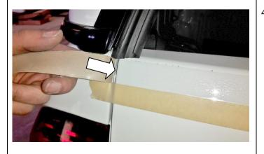
4.13) Push out bubbles and wrinkles as the tape is being laid down, working from one end of the tape with a squeegee.
