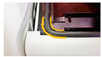
3.7) Apply neutral cure silicon to edge of the bed seal around the front corners both inside and outside of the seal. Clean off excess with a rag applied sparingly with silicon remover or wax and grease remover carefully.
