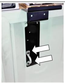
2.14) Bolt the rear corner brackets (3759698R&L, L is shown opposite) to the lower tie down hook mounting points in the tub. Insert 2 off M8x25mm Torx bolts (6151625) through the retained tie down hook, through the bracket and into the tub. Ensure the top bracket tags engage to top of the sides of the vehicle tub. Do bolts up to 22Nm.
