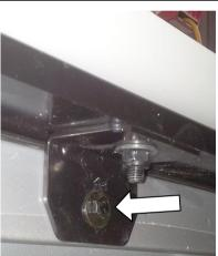
4.5) Apply rust inhibitor to the holes. Fit M6 x 20 mm hex bolts, M6 x 20mm flat washers through the brackets and on the inside secure with M6 wizzlock flange nuts. **Do these up to 9Nm.**
