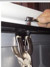
4.3) Locate the slots in the base rail on the inside of the canopy (2 places). Clamp bracket (668PD056) up to the tub lip aligning the top hole in the base rail of the canopy. Apply an M8x25mm hex bolt with M8x20mm washer down through the hole in the top of the base rail. Apply M8x20 washer and nyloc nut up from underneath and do up to 22Nm. Do this in both places on both sides of the vehicle.
