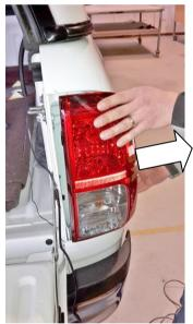
5.1) Pull the light outwards to the side of the vehicle to disengage it from the tub.
