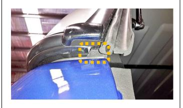
4.10) With the tailgate down and door open, apply neutral cure silicon up into the rear corner tailgate sealing bracket areas, between the tub and the door frame and canopy base rail, to fully seal. Clean up excess and smooth the silicon down on the inside of the canopy.
