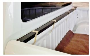
2.2) Apply masking tape over the rail to hold it in place to the front of the tub ensuring the gaps at the ends are even to each side of the tub.
