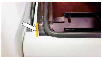
3.6) Apply neutral cure silicon to the ends of the rubber bridge extrusions and seal down the front side of the corner of the tub. Clean off excess with a rag applied sparingly with silicon remover or wax and grease remover carefully.
