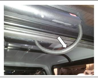
5.18) Fit the second piece of retained 7mm split convoluted tube to the wires between the brake lamp and the interior lamp on the rear door.
