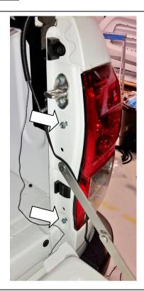
5.0) Undo the 2 screws holding the rear tail lamp assembly to the rear of the tub on the right hand side.
