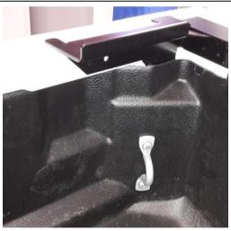
7.9) Clean the front wall of the tub with Isopropyl alcohol for 50mm below the lower edge of the "T" section front rail extrusion all the way along. Fit the bed liner by lifting it up at the rear to snap the side walls of the bed liner in under the side tub rails. Fit the tie down mounting hooks using the original OEM bolts from the tub and **do these up to 22Nm**. Fit the front rail extrusion as per the bed liner fitting instructions. The completed fit should look like the picture opposite.
