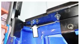
4.7) Insert the rear tub corner sealing brackets (LH shown) into the rear corners of the canopy down on the top face of the canopy's side base rail. Insert M6x20mm hex bolts with M6x20mm washers down through the holes in the top of the bracket through the canopy's base rail. Apply M6x20 washers and M6 nyloc nuts up from underneath. Push the bracket towards the rear of the vehicle with the tailgate closed, to put pressure on the foam tape pad. Do up the bolts to 9Nm in 2 places per bracket.
