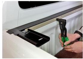
2.12) Remove the masking tape and install 4 rivets (6609087) to the "T" section to assemble it to the front tub panel.
