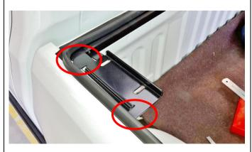
3.3) Apply the seal along to the front bracket at an even offset to the inside of the tub from the rear bracket tags, applying firm pressure to wet out the double sided tape. Ensure the seal inner edge is aligned to the touch the tabs on the front corner brackets on the inner edge.
