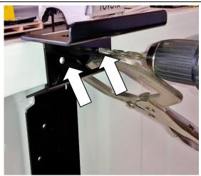
2.15) Clamp the rear tub mounting bracket to the side of the vehicle's tub lip. Ensure the bracket is pushed down so the bumpons on the underside of the bracket engage to top of the side vehicle tub rails. Drill 6.5mm holes through the existing holes at the top of the brackets where they mate up to the lip on the vehicle's tub\_Remove any swarf. Apply rust inhibitor (665505) to the holes.
