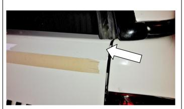
4.12) Starting at the edge of the tailgate, roll out the clear protection tape (665037) and start partially by removing the tape backing liner as small section at a time.
