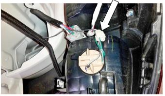
5.4) Apply a 10 meter length of 10mm diameter split convoluted tube (not supplied) to the rest of the canopy's wiring and insert it through the base of the tail lamp recess in the vehicle's tub, through underneath the vehicle.
