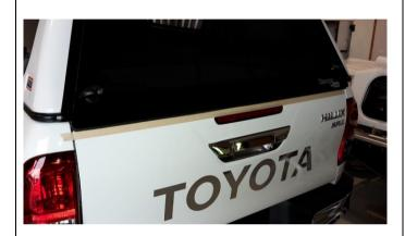
4.11) Apply masking tape to the vehicle's tailgate level with the door's lower glass edge.
