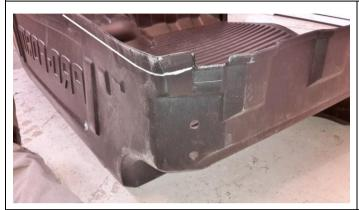
7.2) You will need to trim the bed liner to provide clearance to canopy mounting brackets in the vehicle tub. The following steps are based on fitment to the ARB under rail bed liner. This is based on fitting a new bed liner. (ARB bed liner P/N: KUL3281)
