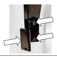
7.7) Complete step 2.3 first. Ensure the bed liner kit's front corner brackets are mounted over the canopy front corner tub mounting brackets. Place the M8 x 25mm Torx bolts (6151625) from the canopy hardware kit though the bed liner front corner bracket (with no washers) on top of the canopy front corner tub mounting bracket. Ensure bolts holding the lower end of the front corner bracket are tightened to 22Nm.
