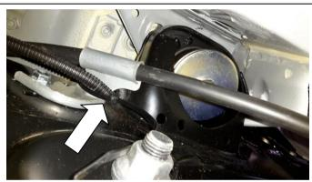
5.10) Cable tie off the wiring loom with 200mm long cable tie near the tray body mount chassis rail bracket.
