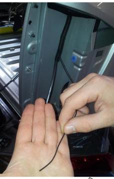
5.3) Cut the end of the thin black wire with white dashed lines from the canopy back to the sheathing. Apply the scotch lock (180701) between the thin black/ white stripe wire from the canopy and the **Green/White stripe wire** on the vehicle's tail lamp.
