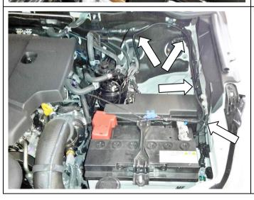
5.14) Pass the wiring loom up the firewall behind all vehicle wiring and piping. Avoid tying to brake lines, AC unit pipes etc, and avoid proximity to exhaust systems and moving parts. Tie off with 200mm cable ties in 4 places as shown to the main vehicle wiring loom in the left hand rear corner of the firewall.
