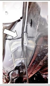
5.11) Cable tie off the wiring loom with 200mm long cable tie near forwards of the rear wheel to the bracket mounted to the chassis rail. <a href="Take care to avoid brake lines and proximity to exhaust systems">Take care to avoid brake lines and proximity to exhaust systems</a>
