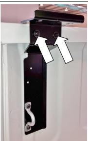
2.16) Fit M6 x 20 mm hex bolts (6151213) with M6 x 20mm flat washers (4591082) under their heads through the bracket holes and on the inside secure these in place with M6 wizzlock flange nuts (6151173). **Do these up to 9Nm.**
