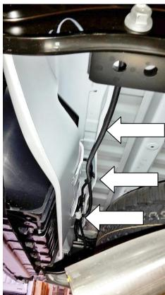
5.6) Cable tie off the wiring loom with 200mm long cable ties to the vehicle's loom across the rear of the vehicle in 3 more places travelling to the left hand side of the vehicle.
