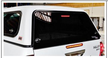
6.0) Depress the vehicle's brake pedal and have a second person check that the brake light works in the door.
