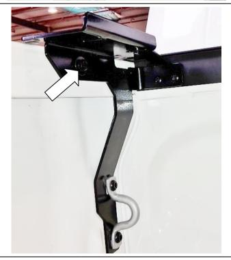
2.8) Fit an M6 x 20 mm hex bolt (6151213) with M6 x 20mm flat washer (4581082) under it's head through the bracket holes and on the inside, secure these in place with M6 wizzlock flange nuts (6151173). **Do these up to 9Nm on both sides of the tub.**
