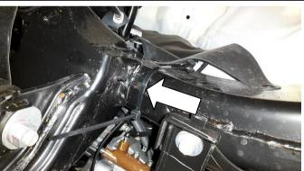
5.13) Towards the engine bay and under the splash shield, rear of the LH front wheel, cable tie off the wiring loom with 450mm long cable ties doubled up (2 required) to the chassis rail under the splash shield. Take care to avoid brake lines and proximity to exhaust systems.
