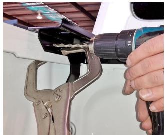
2.7) Clamp the front corner bracket (LH shown) to the side of the vehicle's tub lip in the front corner. Ensure the bracket is pushed down so the bumpons on the underside of the bracket engage to top of the side vehicle tub rails. Drill a 6.5mm hole through the exiting hole in lower bracket corner on the side tub wall with a 12mm deep drill stop fitted. Remove any swarf. Apply rust inhibitor (665505) to the drilled hole. Repeat on other side of tub for the opposite bracket
