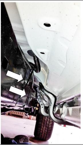
5.12) The picture opposite is looking rearwards down the LH chassis rail. Cable tie off the wiring loom with 450mm long cable ties doubled up, (6 required). Apply in 3 places along the chassis rail. <u>Take care to avoid brake lines and proximity to</u> exhaust systems.
