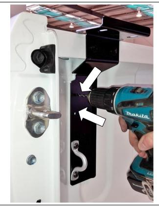
2.17) With a 12mm drill stop fitted, drill 5.2mm holes through the 2 holes in the middle of the rear brackets. Remove any swarf. Apply rust inhibitor (665505) to the holes.
