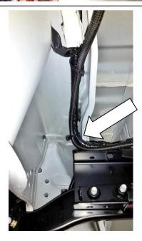
5.7) Cable tie off the wiring loom with 200mm long cable tie to the vehicle's loom along the LH chassis rail rear corner.
