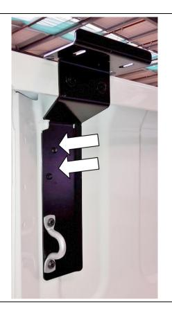
2.18) To the rear brackets, assemble 2 rivets (6609087). Repeat on other side of tub for the opposite bracket
