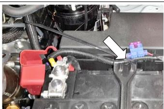
5.16) Fit a 200mm long cable tie around the canopy loom to the battery strap bracket.
