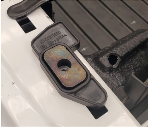
"R" LOCATOR AND SPACER POSITION AT REAR OF TUB
