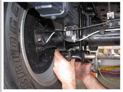
Fit fish plate and secure with flat washers and deep nuts.
