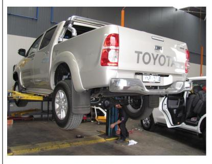
Lift vehicle on hoist. If you do not have a hoist, use a trolley jack.
