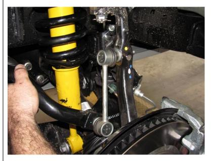
When both left and right hand sides have been fitted, refit and tighten sway bar links and saddles.
