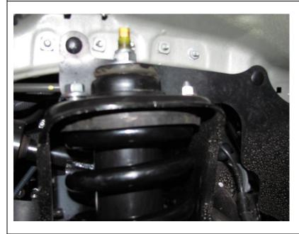
Hold strut assembly in place with one or more nuts secured finger tight.
