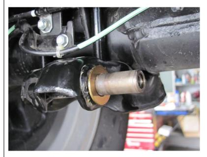
Fit spacer washer supplied with shock absorber behind original factory washer as described by instructions supplied with shock absorber.
