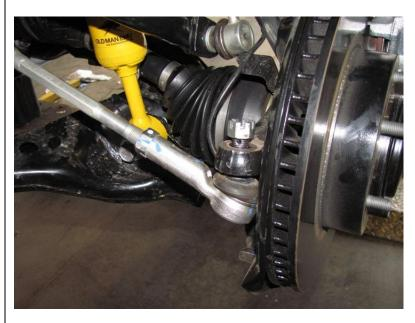
Fit and torque ball joint nut to manufacturer's specification. Secure with split pin.
