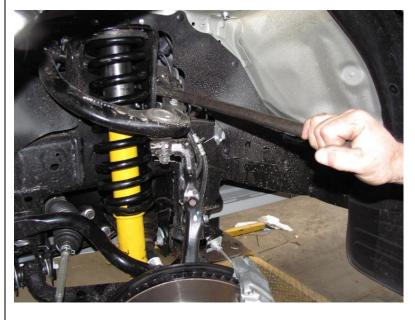
Use a lever bar as shown to aid alignment of the bottom mount in the arm.
