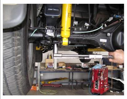
Repeat the entire process to remove and refit the leaf spring assembly on the other side of the vehicle.
