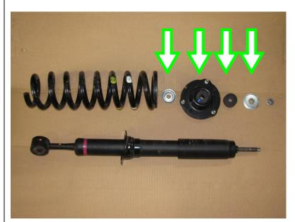
Note components that make up the OE strut assembly.
