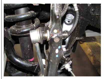
Remove sway bar nut and remove link from mount.
