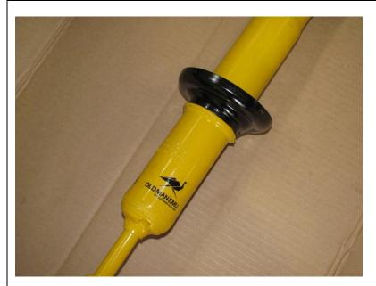
Fit the coil seat to new Old Man Emu shock absorber as shown.
