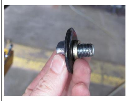
For top and bottom mount fit small spacer to shock absorber mounting bolt as shown.
