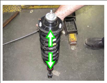
Note alignment of studs on top hat and eye direction. Mark front position with Paint marker
