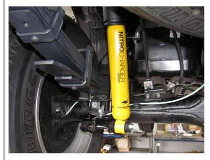
Fit shock absorber and remaining bushings. Secure to manufactures torque specification.
