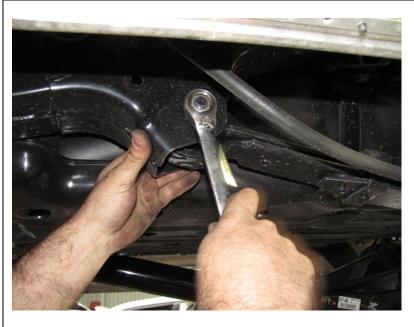
Loosen spring front eye bolt.
