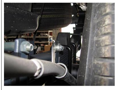
Refit hand brake cable bracket to leaf spring clip.
