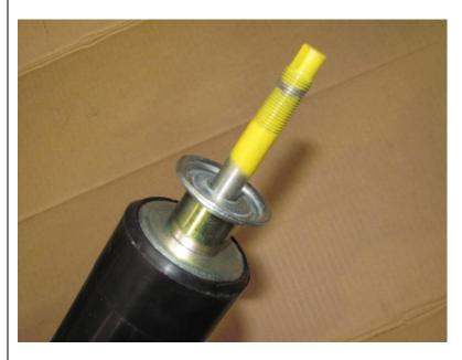
Fit the OE washer to the top shaft of the new shock absorber as shown.
