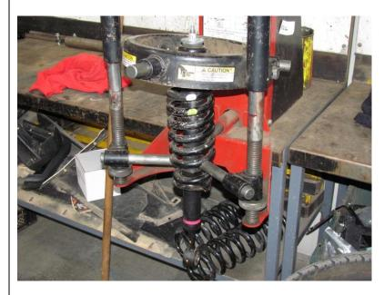
Using a spring compressor disassemble the strut assembly.
