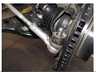
Remove split pin and nut that secures front steering arm ball joint.
