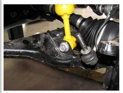
Secure with OE nut and bolt finger tight.
