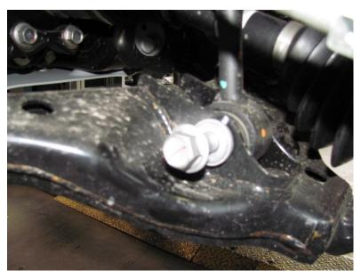
Remove nut that secures damper to bottom arm.
