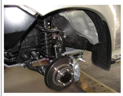
Raise front of vehicle and remove front wheels.
