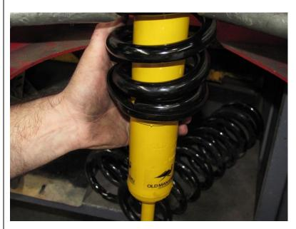
As you unwind the spring compressor align spring seat with the end of the coil.
