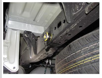
Remove original bushes from chassis. Use pry bar to aid removal if necessary.
