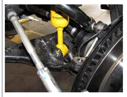
Using the lever bar in the top arm and screwdriver in the bottom eye, align the bottom mount.
