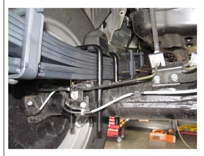
Locate spring centre bolt in axle and refit factory bump stop with Old Man Emu U bolts.
