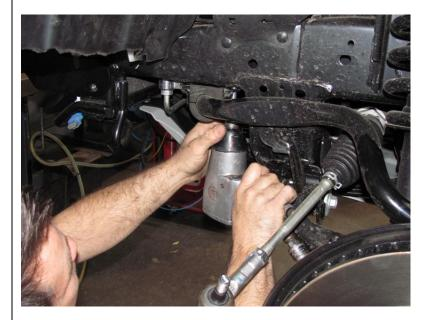
Remove sway bar saddle bolts. Rest sway bar on under vehicle splash pan.
