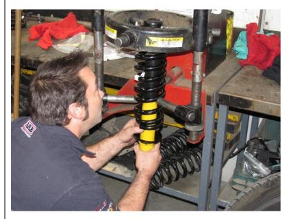
Compress spring such that the damper can be pushed home against the top hat without the spring seat coming up to contact the bottom of the spring.
