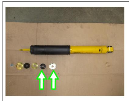
Noting correct position of new shock absorber hardware, fit retainer washer and bushing as indicated to shock absorber top shaft.
