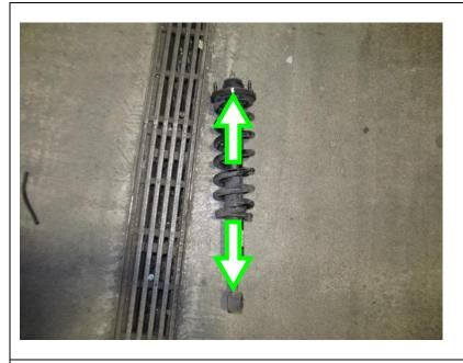
Note alignment of studs on top hat and eye direction. Mark eye position with paint marker.
