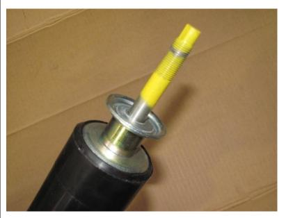
Fit the OE washer to the OME damper as shown.
