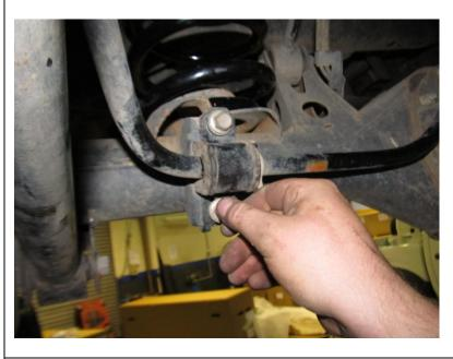
Replace sway bar saddle bolts and torque to manufacturer's specification.
