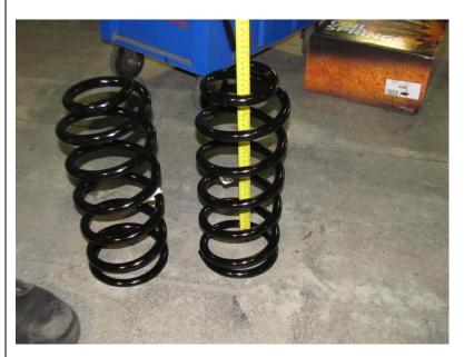
Before fitting measure and note free height of both left and right hand springs.
