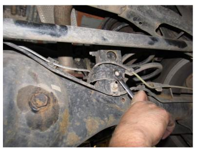
Remove brake line and ABS sensor cable retainer brackets from the axle housing.
