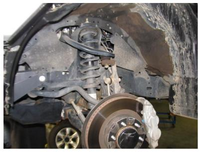
Raise front of vehicle and remove front wheels.
