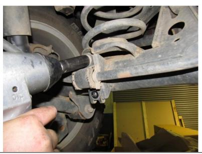
Remove rear sway bar saddle bolts. Once removed let unhook saddles from axle and let sway bar sit on top of differential housing away from rear axle.
