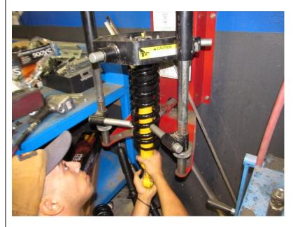
Compress spring such that strut can be pushed all the way into the top hat without the spring touching the spring seat.
