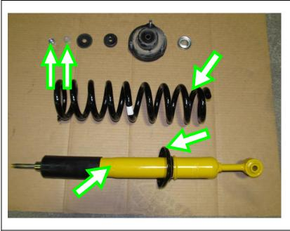
New Old Man Emu parts supplied are the damper, spring, spring seat, top nut and washer.
