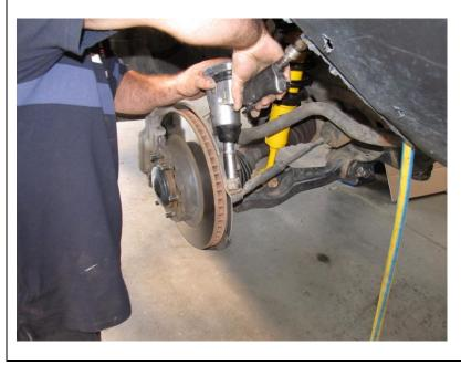
Fit and tighten ball joint nut.
