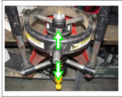
Align damper bottom mount and top hat studs as per OE.
