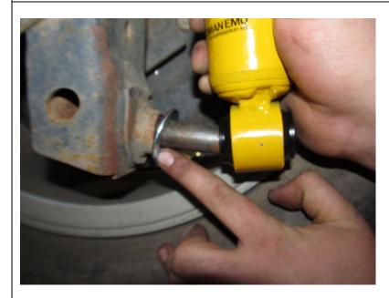
Install new washer from Old Man Emu shock absorber on bottom shock absorber mount.
