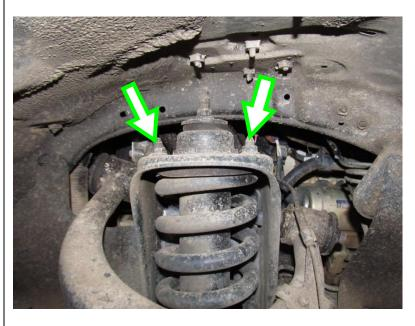
Tools: 14mm ratchet spanner 14mm socket and torque wrench
