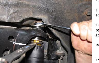
Tighten using 19mm spanner.
