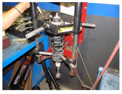
Tools: Strut compressor 17mm spanner 8mm spanner
