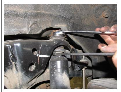
Before raising vehicle, loosen the top nut on the rear shock absorber. Prevent shock from spinning by using 19mm spanner on the flat section below the top stud.
