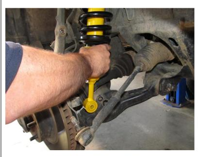
Use a lever bar in top arm as before to aid alignment of the bottom strut mount in the lower arm.
