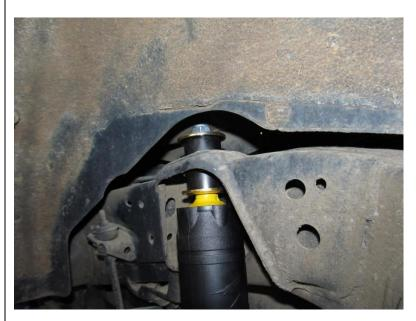
Lower vehicle to partially compress suspension.
