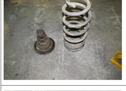
Fit factory bump stop to new Old Man Emu spring in original position as shown.
