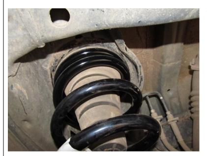
With another person's assistance, whilst slowly lowering vehicle, relocate spring to spring seat in original position.
