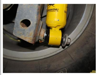
Compress new Old Man Emu shock absorber and fit to the bottom mount.
