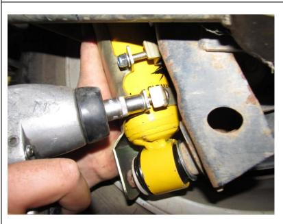
Align stone shield to cover the front of shock absorber. Ensure that lower mount bushing and washer is completely covered.
