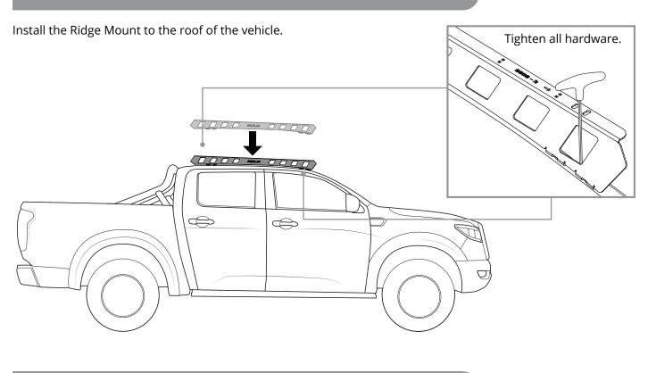
Install the Ridge Mount to the roof of the vehicle.
