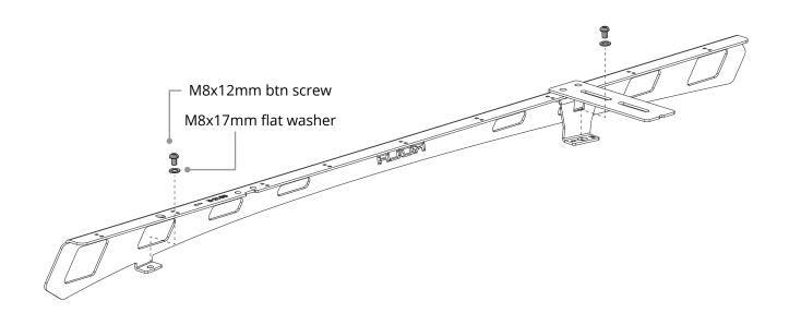
Place the Ridge Mount assembly onto the roof. The M8 hardware will pick up the exposed anchor points in the ditch.
