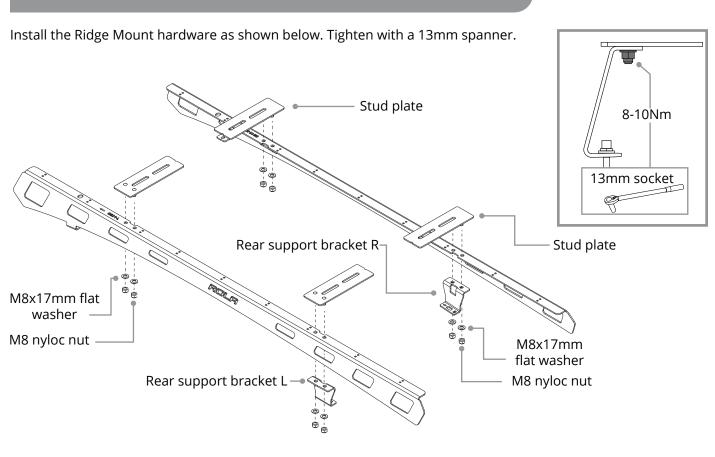
Assemble M8 mounting hardware into the Rails as shown.
