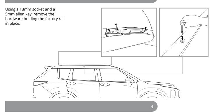
Carefully remove the factory rails, cleaning the roof ditch when done.
