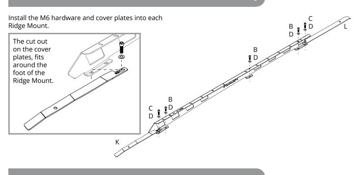
Place the Ridge Mount assembly onto the roof. The M6 hardware will pick up the exposed anchor points in the ditch.
