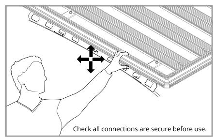
Wiring can be run and secured on the underside of the Ridge Mount rail as shown.
