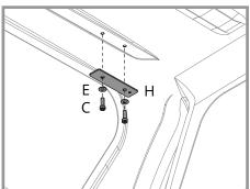
From the inside of the canopy, slide the M8 hardware through the mounting plate, up through the canopy and into the Ridge Mount above.
