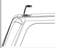
Set the Ridge Mount 27mm forward, of the rear of this detail.
