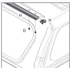
From the outside of the canopy, slide the M8x20mm screw and washer, through the Ridge Mount and canopy. Fix from the inside with the accessory bar and nyloc nuts.
