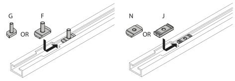
If accessory ports are not available, hardware can be dropped directly if channel width permits.
