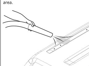
Use a soldering iron and seal the drilled sections of the canopy. This will remove any potential micro cracks from causing issue.
