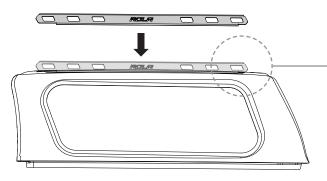
Recommended position: Sit the Ridge Mount into the most outer roof detail. Centre in this detail.
