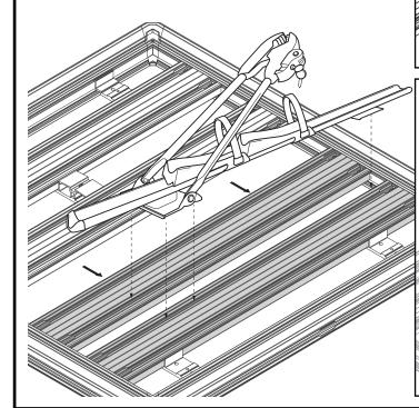
A - Once position is adjusted, slide 2x T-bolts in one channel and a single T-bolt in the adjacent plank.
