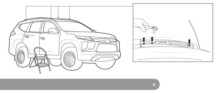
Remove the hardware covers with a trim tool along the rail body. With a 10mm socket wrench, remove the hardware.
