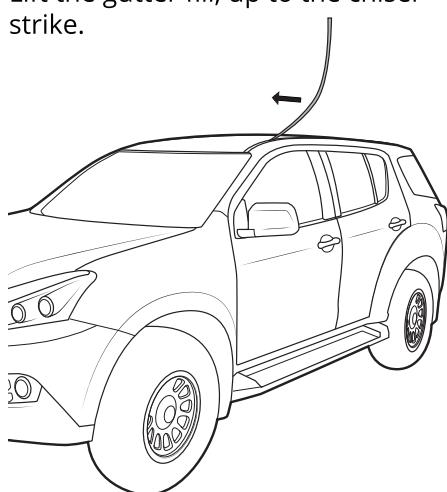
Move the fill back and forth until it breaks free of the vehicle. Use cutters if required.
