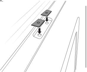
Cut a butyl patch in half, placing a section over the centre hole now exposed, in the mid portal.
