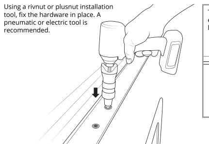
The stem of the plusnut will compress and engage the interior surface of the vehicle, locking the nut in place.
