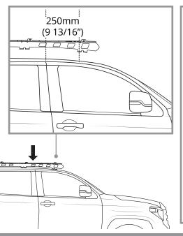
Centre the holes of the Ridge Mount on the gutter.
