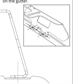
Mark the centre of each mounting hole in the Ridge Mount onto the gutter below.
