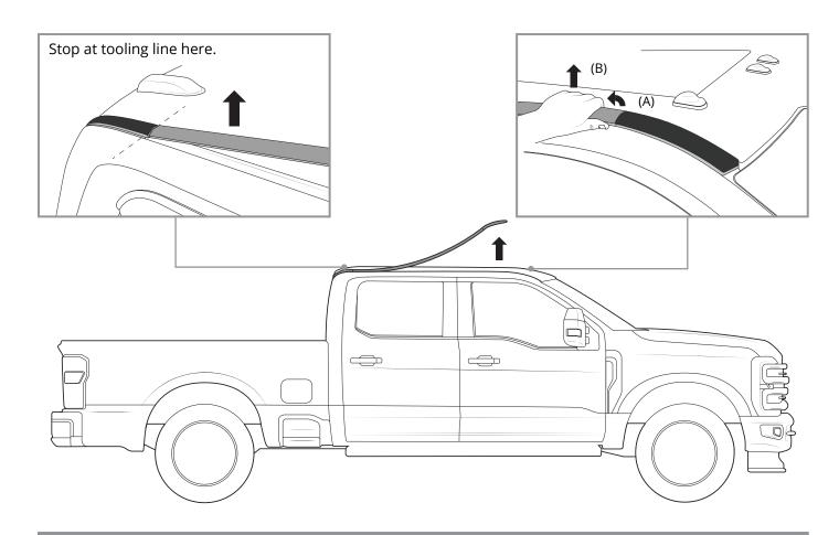
The clips holding the fill may require removal after it is pulled free. The can be done safely with trim tools.
