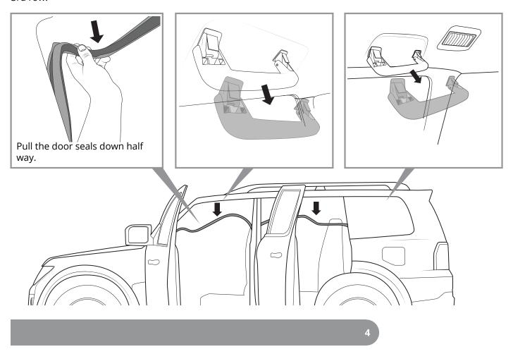
Carefully remove the B-pillar and 3rd row cowling as shown.
