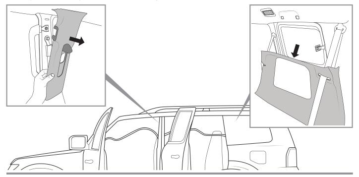
Finally remove the 4x plastic plugs in the roof, allowing the hood lining to come free.
