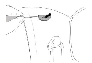
Pry the cover forward slightly, removing its grip from the roof liner.
