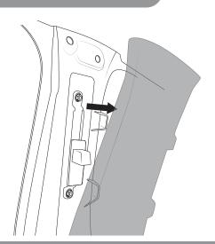
Partially remove the rubber seal from around the upper sections of the door frames.
