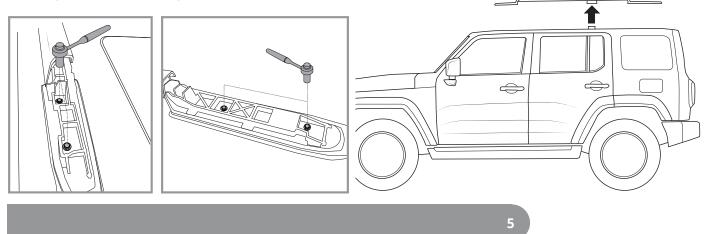
Using a 13mm socket, remove the centre factory bracket. Clean the roof of any debris.
