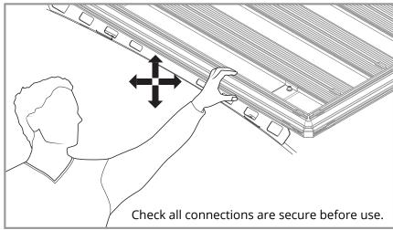
Wiring can be run and secured on the underside of the Ridge Mount rail as
