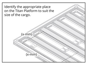
2 Slide a T-bolt into the c-channel of the platform, moving them to dimensions of the previous step.
