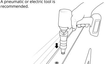
The stem of the plusnut will compress and engage the interior surface of the vehicle, locking the nut in place.
