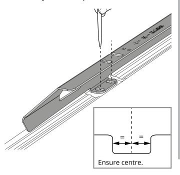
Using a centre punch, make a reference at the centre of the marks just made.
