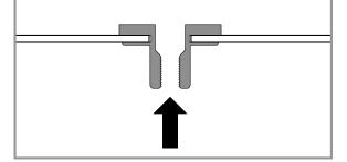
Place the Ridge Mounts back into place. Measure the gaps between the feet of the assembly and front and rear. Cut the ditch fill to these lengths.
