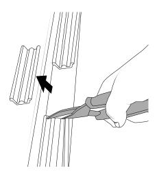
Be sure the ditch is clean of adhesive and debris in the cut areas.
