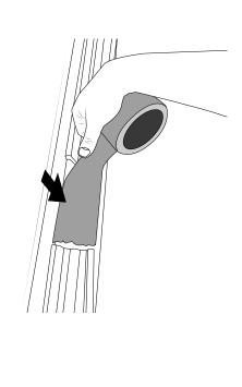
Place the Ridge Mounts into place. Mark all holes in the assembly on to the tape below.
