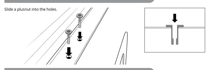
Using a plusnut installation tool, fix the hardware in place.
