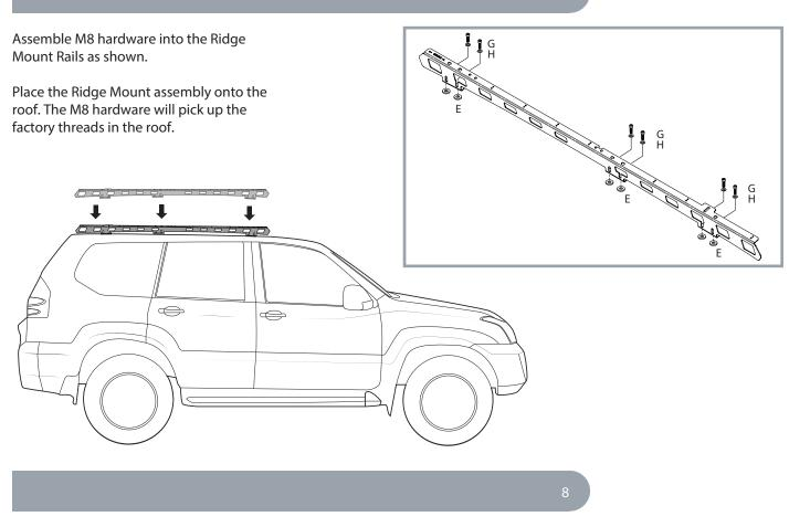
Assemble the stud plates and corresponding hardware onto the system. Tighten in place.
