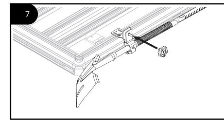
Secure the carried item by tightening with the plastic knobs provided.
