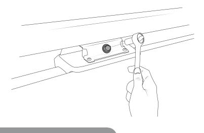
Remove the factory rail from the vehicle.
