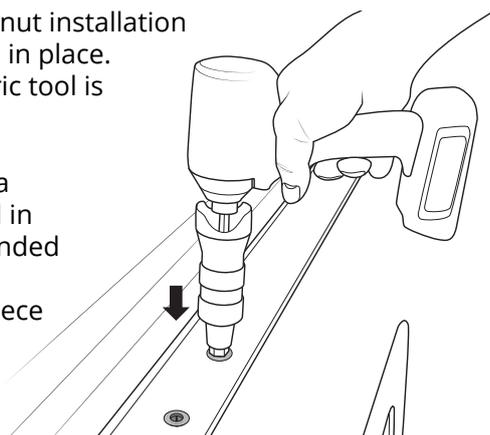
The stem of the plusnut/ rivnut will compress and engage the interior surface of the vehicle, locking the nut in place.
