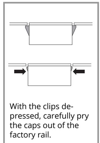
With the clips depressed, carefully pry the caps out of the factory rail.
