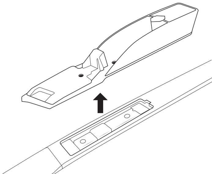
B - Place a base plate into the position over the exposed threads. Be aware of front and rear plates.
