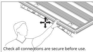
Wiring can be run and secured on the underside of the Ridge Mount rail as shown.
