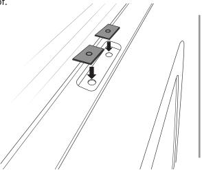
Cut a butyl patch in half, placing a section over the centre hole now exposed, in the mid portal.
