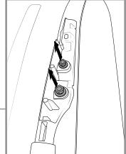
Remove the mid factory rail supports from the roof.
