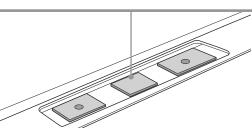
Install the M8 hardware into the Ridge Mounts.
