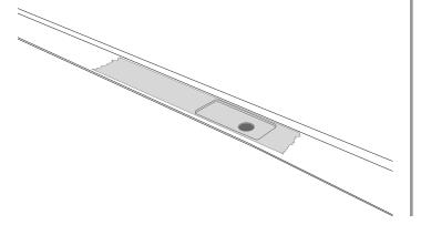
(B) Using a marker, create a reference 130mm toward the rear of vehicle, following the sides of the port as shown. Connect the two lines, creating a rectangle.
