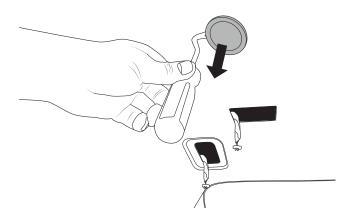
Remove the cover from the speaker by pushing on the corner of the cover.
