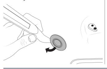
Release the harness to disconnect the light.
