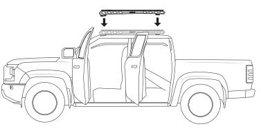
Fix in place with an M8 washer and nyloc nut, on the inside of the vehicle.
