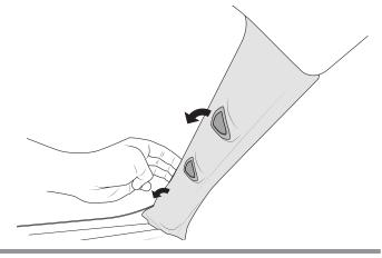
Start to pry the passenger side out in the same fashion. Once the side of the cover is released, pull the cover along the A-pillar. This will clear the clip holding the cover at its top end. Remove the cover.
