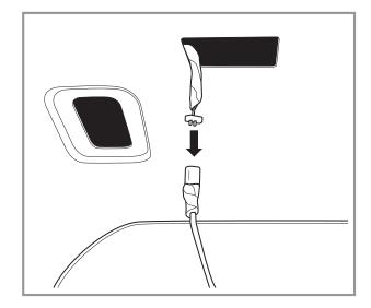
Remove the A-pillar handle by prying on the bottom edges of the handle covers. This will expose the hardware below, remove to detach the handle.
