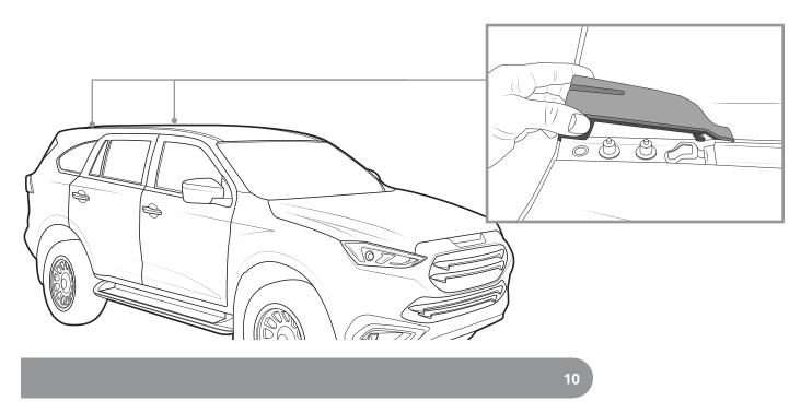
Using a flat blade screwdriver, carefully lift the ditch fill from the rear of the vehicle. Roll the fill forward to the cut made step 8. Remove the fill.
