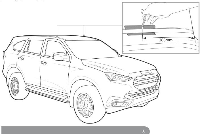
Using a dremel, cut through the ditch fill at the reference made previous.
