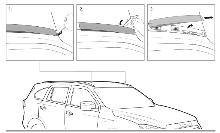
Using an appropriate trim remover tool, carefully wedge the rear of the rail covers upwards to release the internal clips. Release the clips on the inside edge of the cover in the same manner.
