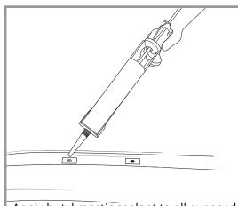
Apply butyl mastic sealant to all exposed M8 threads.
