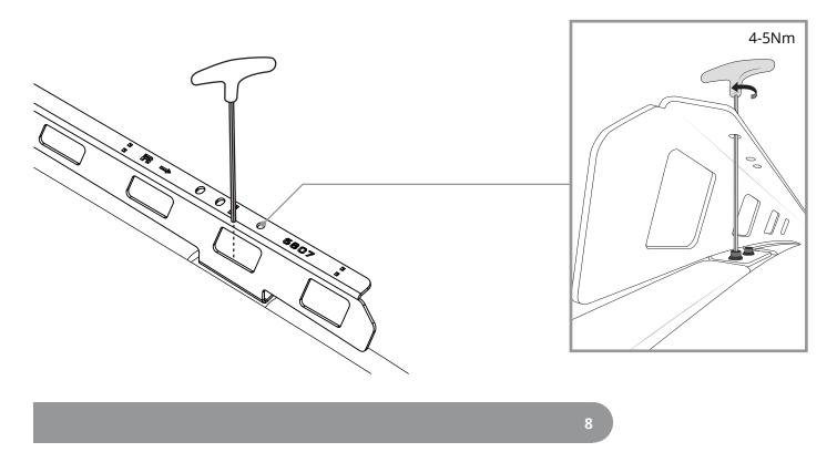
Assemble the stud plates and corresponding hardware onto the system. Tighten in place.
