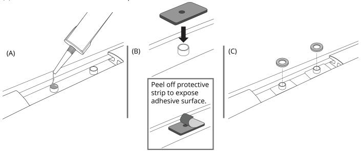
Assemble M8 hardware into the Ridge Mount Rails as shown.
