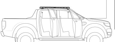
Use the factory nuts to fix the Ridge Mount down.
