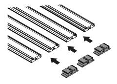
Install the interlocking blocks, as per step 6 in the Titan Tray Fitting Instructions.
