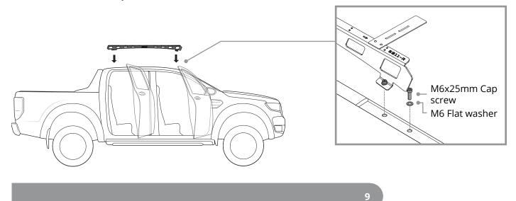
Fix the Ridge Mount assemblies in place, using the factory nuts removed in step 3. Assistance will
