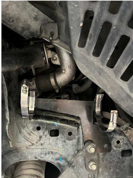
Once this is complete, the shock can be inserted into the tower and bolted in. Make sure that the hose from the the top of the shock is pointing to the front of the vehicle for reservoir positioning and that the lower mount rebound adjuster is facing the front of the vehicle. Once shock is mounted, the reservoir canister can be inserted and hose clamps tightened. Below is the recommended position of the canister
