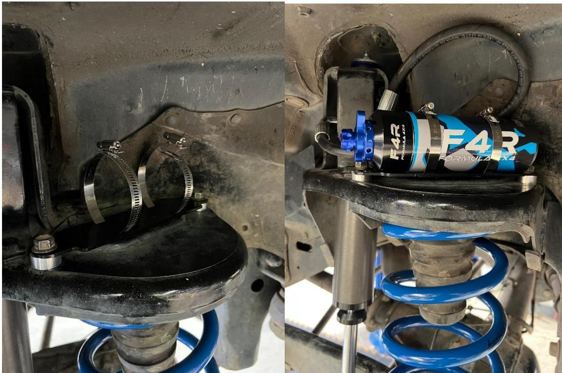
Once installed, attached all removed parts to complete front install.
