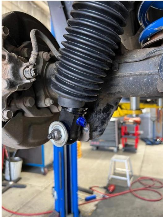
The positioning the hose and reservoir may need to be adjusted to suit fitment in vehicle. Please see suggested images below on fitment. To realign, simply undo the bolt holding the clamp and place reservoir as need. The reservoir is on a swivel hose, so can be inverted if necessary. It is always recommended to fit shock before spring and jack each side up to full bump to ensure no contact is made with the reservoir positioning.
