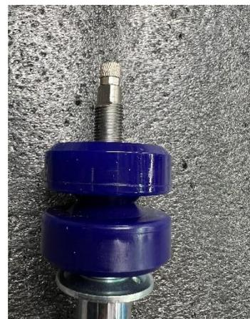
Due to the heavy-duty design of the damper, it may be required to turn the adjusters one or two more clicks anticlockwise in compression and rebound for the first couple of thousand km, to reduce the stiffness and account for a running in period. Please make is full adjustment range on clickers before install as they may be stiff from assembly.
