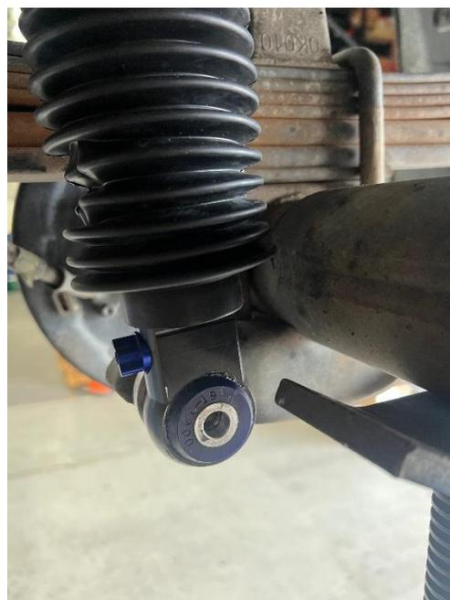
The positioning the hose and reservoir may need to be adjusted to suit fitment in vehicle. Please see suggested images below on fitment. To realign, simply undo the bolt holding the clamp and place reservoir as needed. The reservoir is on a swivel hose, so can be inverted if necessary. It is always recommended to fit shock and articulate vehicle to ensure no contact is made with the reservoir positioning.
