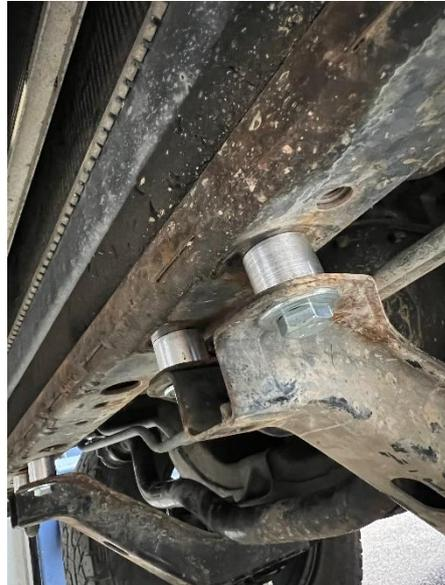
With previous shock removed, Swaybar unbolted from the links and mounting point, insert the two relocation plates to sway bar mounting point with reservoir bracket in between. Once relocation plate is in position remount sway bar to plate.
