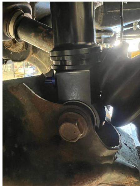
Once shock is mounted, the reservoir canister can be inserted and hose clamps tightened. Below is the recommended position of the canister
