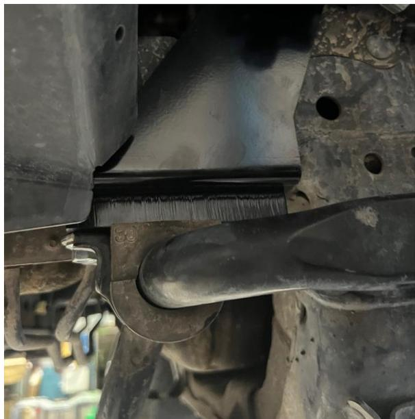
Once this is complete, the shock can be inserted into the tower and bolted in. Make sure that the hose from the the top of the shock is pointing to the front of the vehcile for reservoir positioning. Ensure that the lower shock mount has the rebound adjuster pointing inwards.
