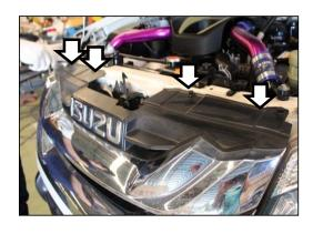
Then remove OEM Plastic radiator cover attached to the top of grille.
