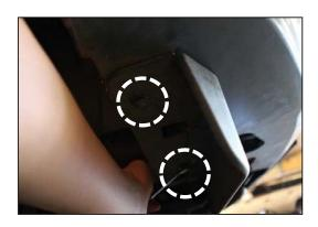
Remove and keep for re-fitment two original nuts that retain the bumper at the bottom
