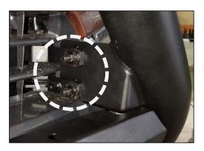
19 Fully tighten the Chassis Mounting Bolts. by using four M10 Socket head (M10x35x1.25), spring washers, flat washers and M10 flange nut.
