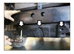
Remove and keep for re-fitment three original bolts from the lower plastic stone tray .
