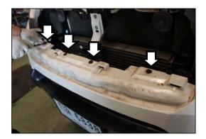
5 Remove the clip and screw retaining the lower edge Keep for re-fitment.
