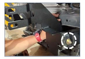
Place LH, RH chassis mount onto the chassis of vehicle and secure by using M10 bolt (M10x1.5x80), spring washer, flat washers and Flange nut.
