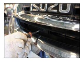
Remove one screw that retain the grille at the front. Keep for re-fitment of grille.
