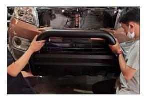
Lift the A- bar fit to the chassis mount ,Align the A- Bar to the desired position.
