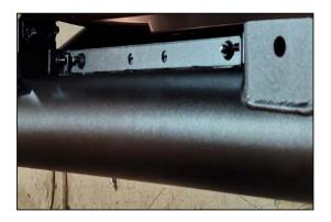
Assemble License plate bracket by using M6 x L 20, M6 Flat washer, M6 Spring washer, Flange nut M6 and fully tighten.
