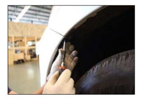
7 Remove and keep for re-fitment the screw retaining the bumper bar in the wheel arch.
