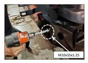
Re-install the cross bar to the Re vehicle by using four M10 bolts (M10x35x1.25), spring washer and flat washer secure through the chassis mount.
