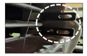
17 Re-install the front bumper and place the chassis mounting bracket through out the bumper as shown.
