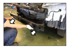
Remove and keep for re-fitment the front intrusion beam from the vehicle.]
