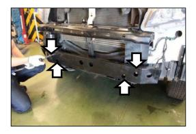
Remove and discard four bolt on intrusion beam as show in the figure.
