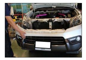
9 Carefully remove the bumper from the vehicle.
