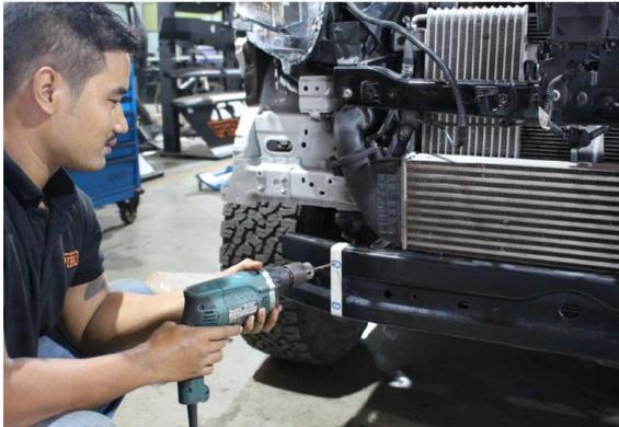
**33** Drill a pilot hole through both sections of the intrusion beam . Using a step drill or similar, enlarge the holes to 18mm. .
