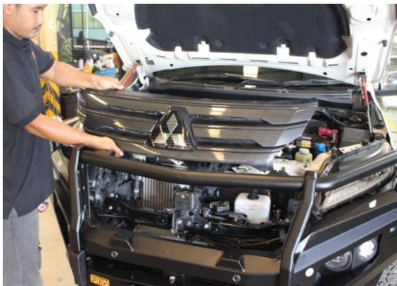
**122** Insert the grille to mark the location for drilling holes in the grille.
