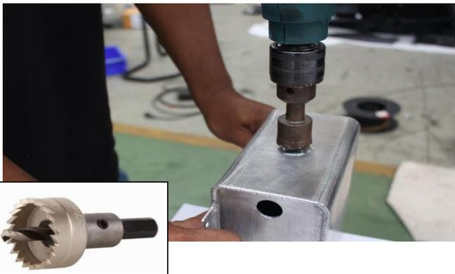
**58** Drill hole use hole saw 30 mm. as shown. chamfering the drilled edge.
