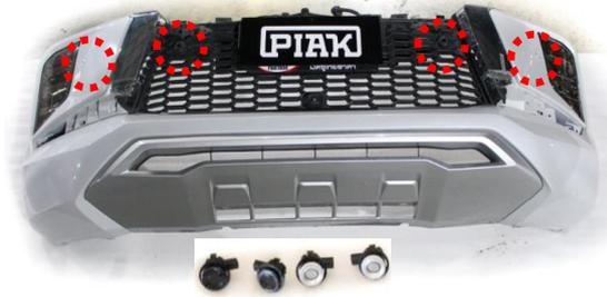
**83** The location of parking sensor loom (where fitted) at the front of bumper bar.
