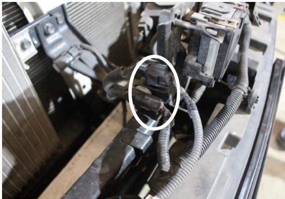
**18** Disconnect power cable and camera located behind grille.
