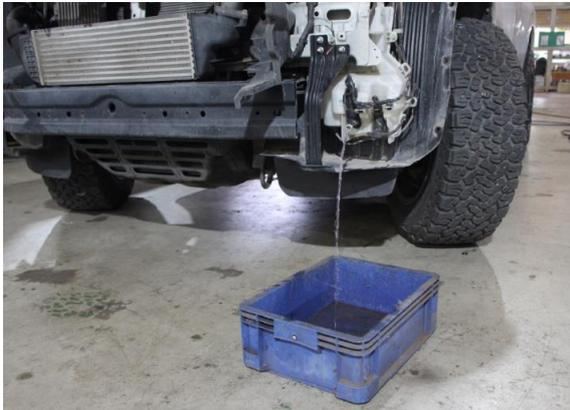
**17** Drain the fluid from the washer bottle.
