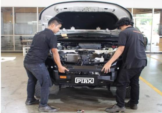
**104** Lift the bullbar onto the chassis of the vehicle.
