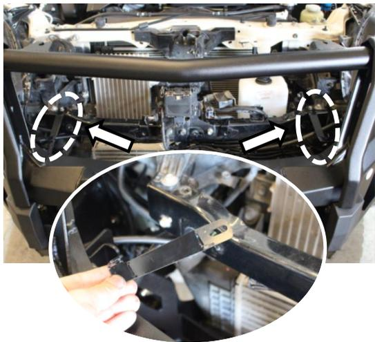
**121** Attach the Front grille bracket to the grille using the tek screws that are at the back of the grille.
