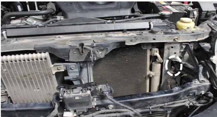
**63** Fix Windshield Washer Bracket A on the body car. Using tow original bolts as shown
