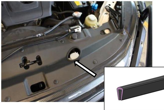
**73** The drilled hole to use for open-close the lid Windshield Washer Bottle.
