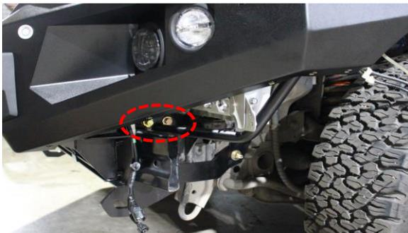
**110** Secure wing support bracket to M10 bolt that fitted the outer mounting bracket by using flat washers and hex nut.
