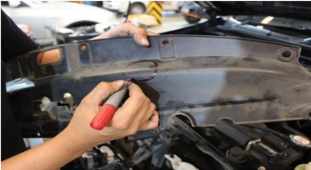
**71** Re-fitment the upper bumper and sketch the circles to match the lid Windshield Washer Bottle for drilling.
