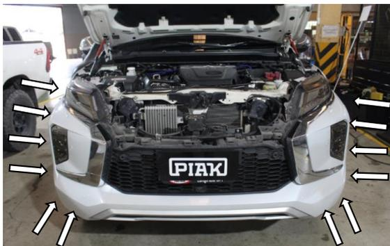
**11** Remove the clips on the fenders and the bolt on the bottom of the bumper.
