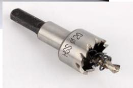
**56** Drill hole use hole saw 20 mm. as shown. chamfering the drilled edge.
