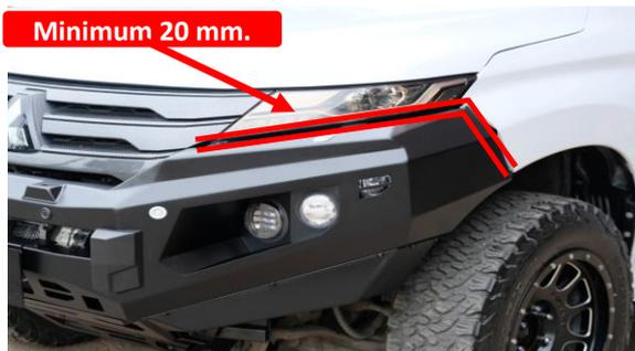
**106** Align the bar so there is a minimum 20 mm. gap between the car and wing return of the bar and the end of the wing is in line with the wheel arch.
