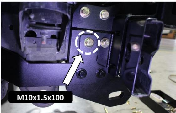
**46** Secure with two M10 bolts (M10x1.5x110), Spring , Flat washers and Hex nuts as shown, both sides of the vehicle.
