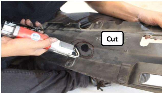
**72** Cut into holes. For opening the lid to put water.
