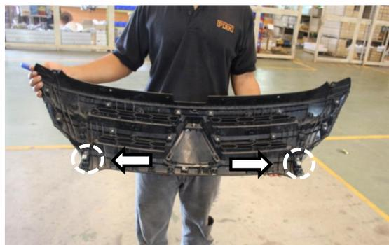
**123** Drilling holes 3 mm. in the grille at location as shown for mounting front grille bracket .
