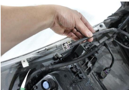
**77** Mark the location of the water nozzles and remove the water line from the water nozzles.
