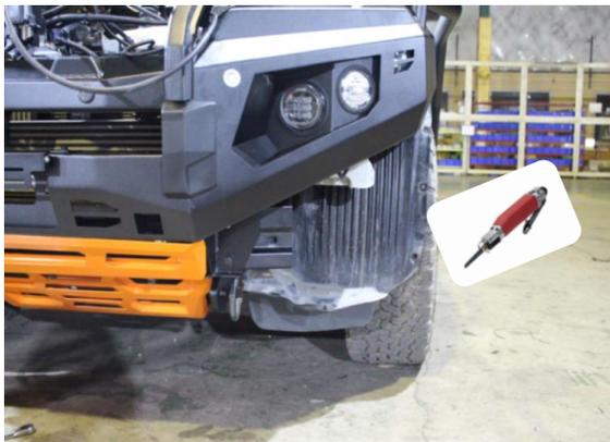
**118** Use a saw to cut off the fenders as shown.
