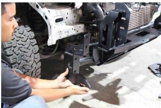
**36** Connect chassis support bracket onto the chassis mount and insert wire bolt through the hole of bracket both sides of the vehicle.
