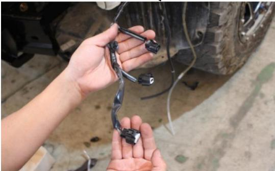
**50** Using wiring harness L850 mm. Connect the motor cable original and Water Sensor taken.
