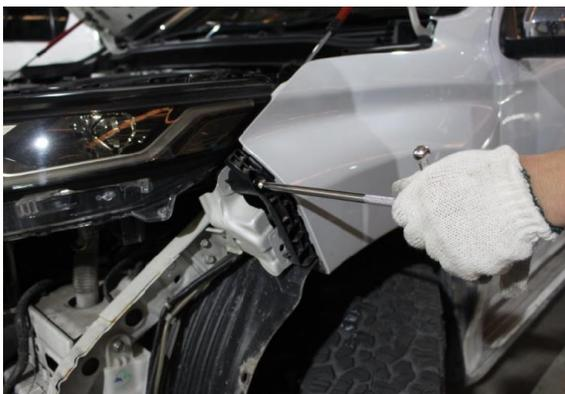
**20** Remove and discard the outer bumper clips from the front guards.
