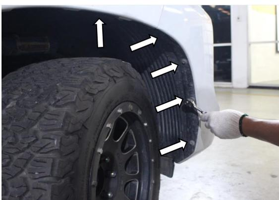
**12** Remove five clips that retain the outer edge of the bumper (Both sides).
