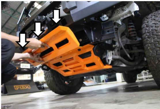
**117** Install the Protection Plate Center 01 on Protection Plate Center 02 on to the under body of car as shown.
