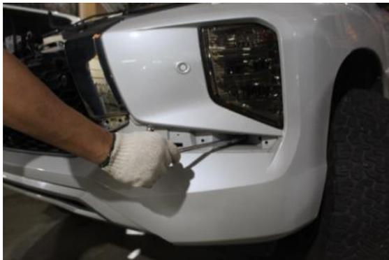
**10** Remove the inner bolts (Both sides).
