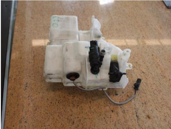
**53** Remove the parts of original windshield washer reservoir as shown.
