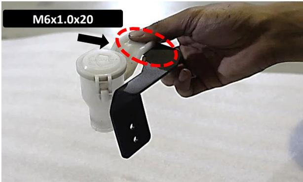
**69** Fix lid Windshield Washer Bottle and on to the Windshield Washer Plate B. Use hex bolt M6x1.0x20 ,Flat washer and Flange nut.
