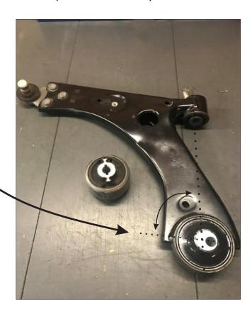
Re-fit arm to vehicle using original bolts.
