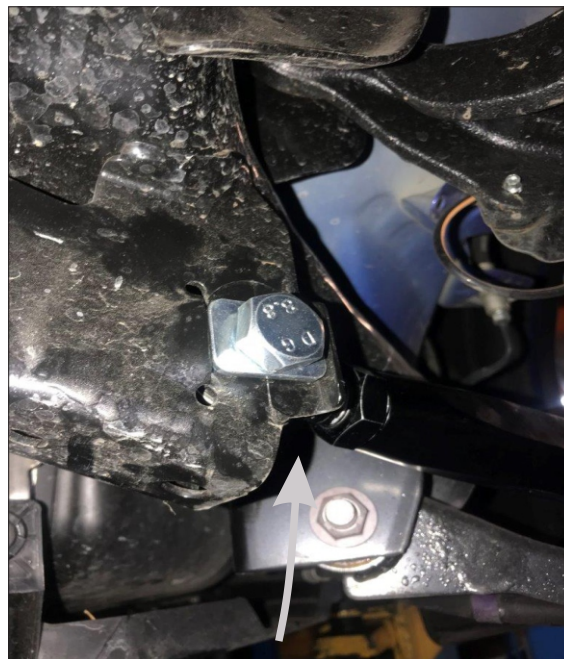
Lock washer and new bolt installed
