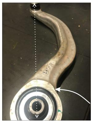
Instructions Front Radius Arm Bushing - Anti-geometry + caster + low compliance
