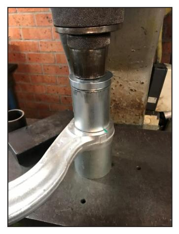
Note - there is a small chamfer on the aluminium arm - to help with press in.
