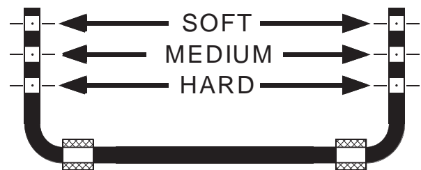
WHITELINE Blade adjustable swaybar - rate adjustment guide
