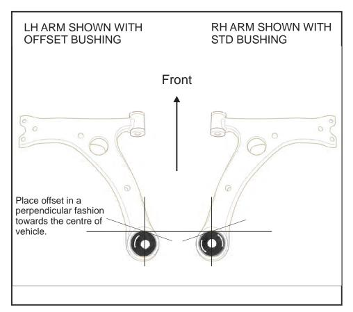
Press bushing in with voiding orientation as per above. Note the offset unit for max caster gain.
