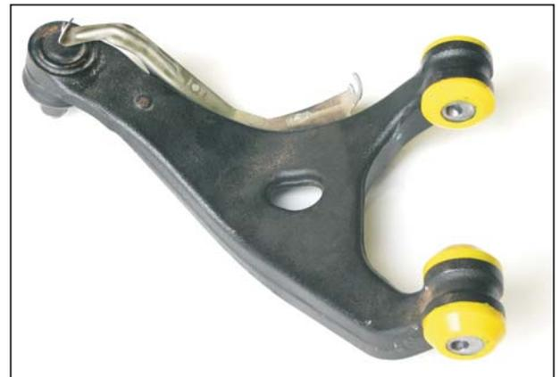
Fig 2 - left control arm with new bushes.
