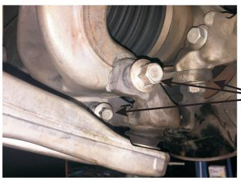
• Un-bolt lower front bushing bolt.
