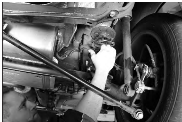
Unbolt lower shock mount and remove coils.
