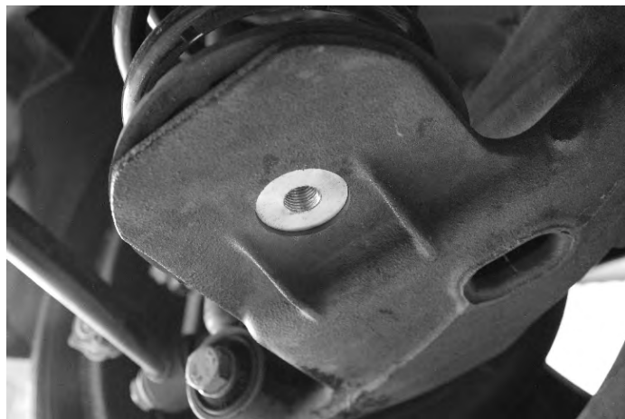
Confirm threaded boss is properly located.
