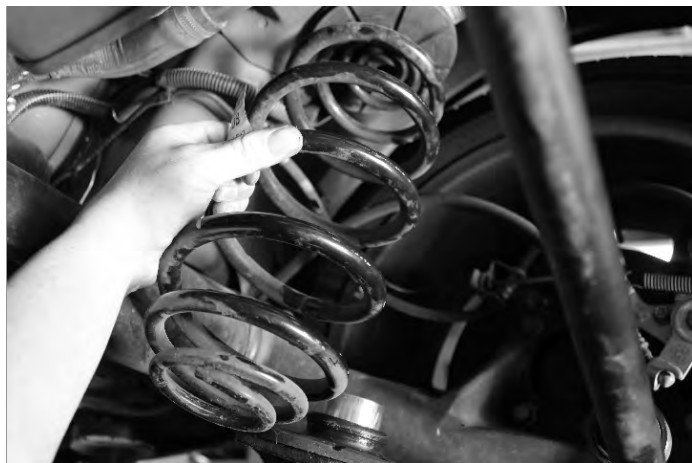
Re fit spring pads and coils
