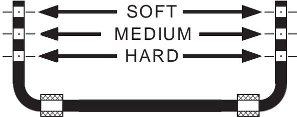
WHITELINE Blade adjustable swaybar - rate adjustment guide
