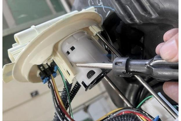
Photo 4: Remove OEM rollover valve
