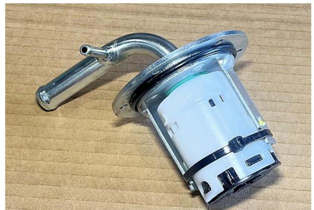
Photo 5: Refit OEM rollover valve
