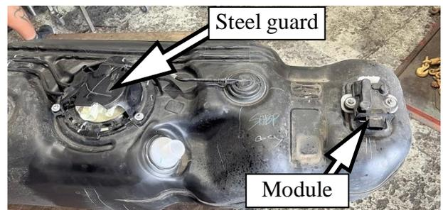
Photo 2: OEM tank preparation
