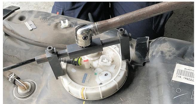
Photo 5a: Remove pickup unit
