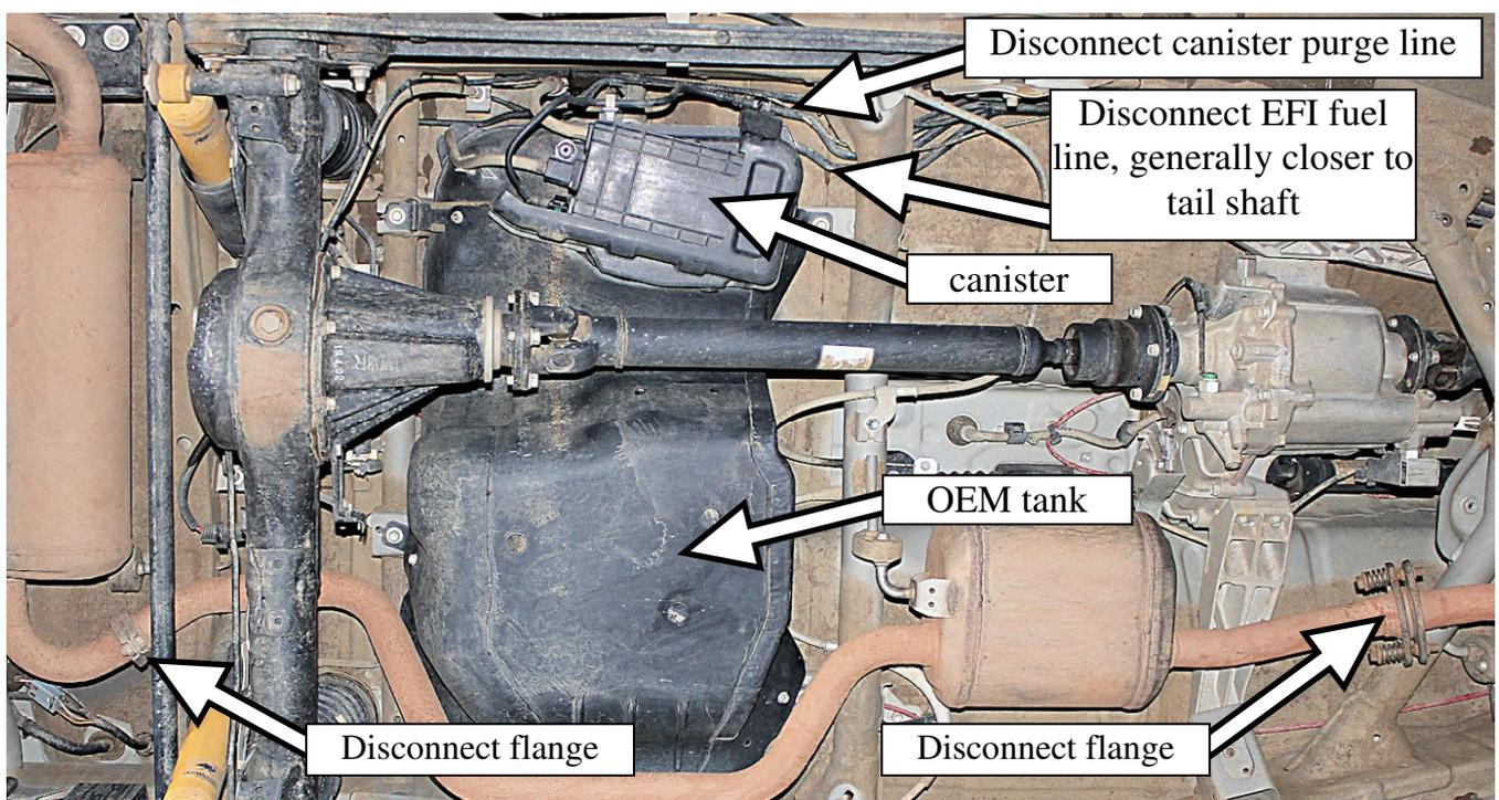
Photo 1: Tank removal preparation
