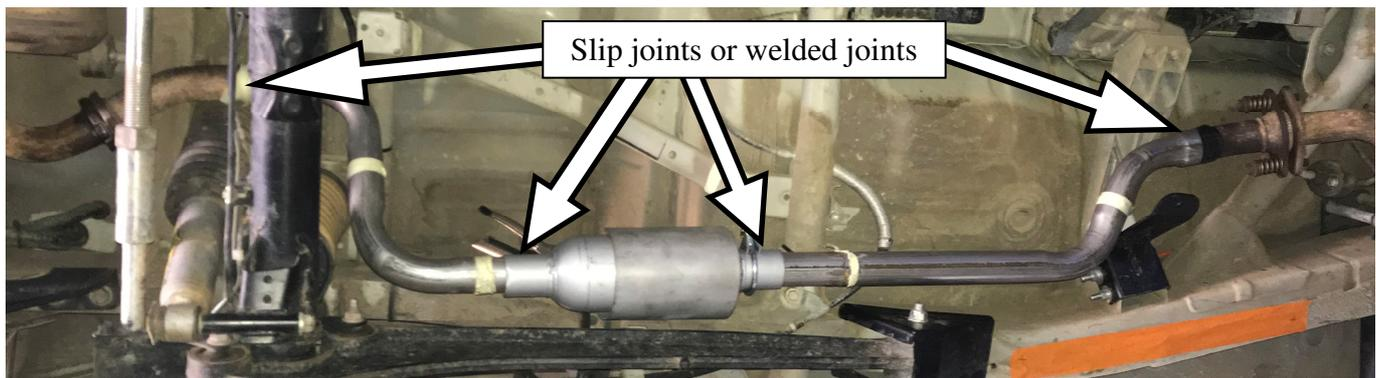
Photo 11: Rebuild mid-section of exhaust with parts supplied
