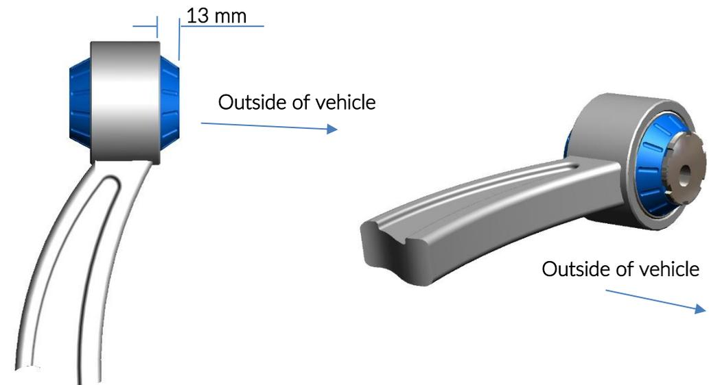
Figure 02 View looking down on left hand arm bushing installed
