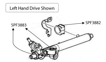
This Kit can be installed without removing the Steering Rack from the vehicle, for best results it is recommended that the Steering Rack be removed to aid installation;
