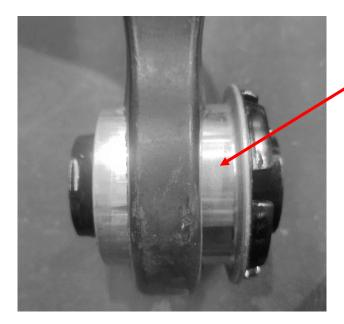
9.5mm gap between the underside of the flange and the highest point on the outer face of the arm (same for both bushes)
